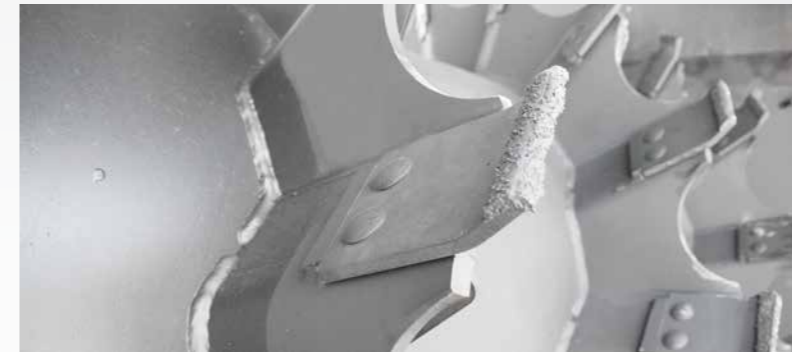
Additional hardening - armoured drum tools
