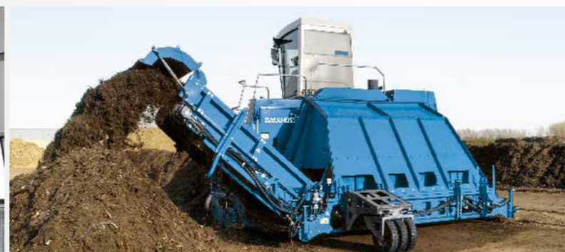
Intelligent space utilization - Side Conveyor
