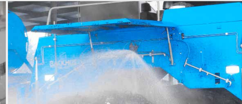
Process optimization - injecting water during turning
